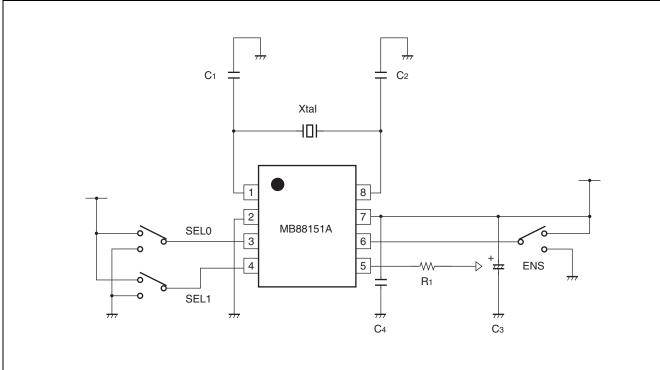
$C_1,\,C_2$  : Oscillation stabilization capacitance (refer to "Oscillation Circuit".)
