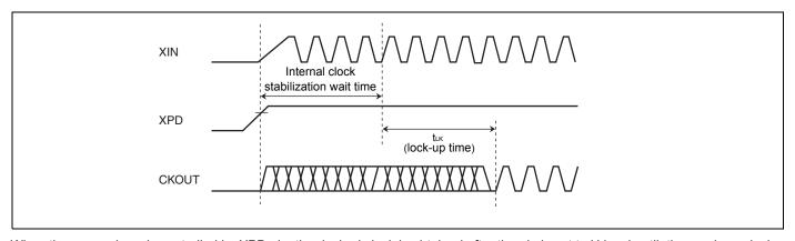
When the power down is controlled by XPD pin, the desired clock is obtained after the pin is set to H level until the maximum lock-up time  $t_{\rm LK}$  is elapsed.
