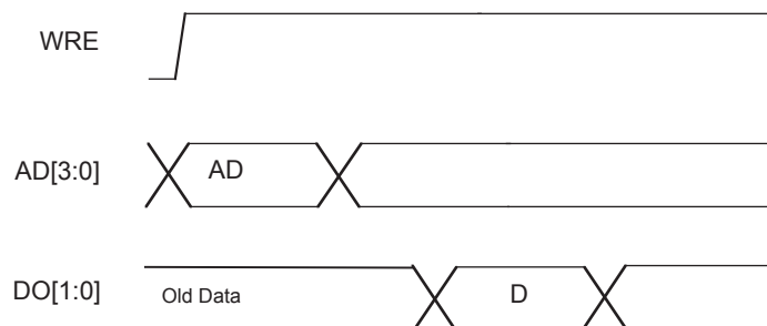
Figure 3-7. Slice Single /Dual Port Read Cycle Timing
