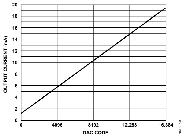
Figure 95. Gain Curve for FSC[9:0] = 512, DAC OFFSET = 1.228 mA
