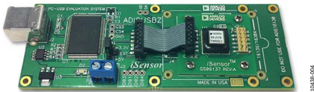
Figure 3. ADIS16265/PCBZ and ADISUSBZ
