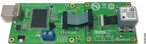
Figure 4. ADIS16210/PCBZ and ADISUSBZ
