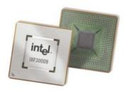
or as strong FEC devices, providing a net electrical coding gain of 10dB in Ultra Long Haul (ULH) or submarine systems.
