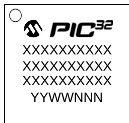
64-Lead QFN (9x9x0.9 mm)
