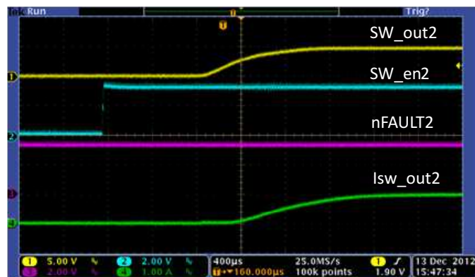
Figure 40. USB Switch2 Start-Up 1A Load
