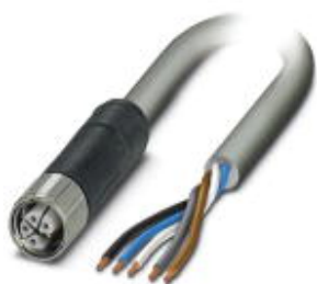
Power cable, 5-position, PUR halogen-free, gray RAL 7001, Socket straight M12, L-coded, on free cable end, cable length: 10 m
