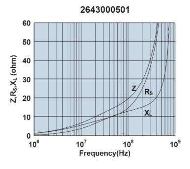
Impedance, reactance, and resistance vs. frequency.
