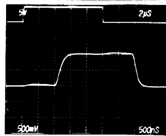
MUX-08 SMALL-SIGNAL SWITCHING WITH FILTERING AND 2.5μs SAMPLE TIME
