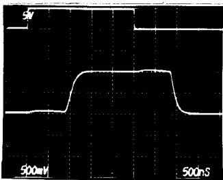
MUX-24 SMALL-SIGNAL SWITCHING WITH FILTERING AND 2.5μs SAMPLE TIME
