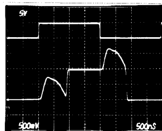
MUX-24 SMALL-SIGNAL SWITCHING WITH 2μs SAMPLE TIME
