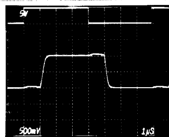
MUX-08 SMALL-SIGNAL SWITCHING WITH FILTERING
