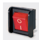
C1553AA with M616 guard Cut-out 22.0/22.1 x 29.4/29.5 Guard accepts "A" body only
