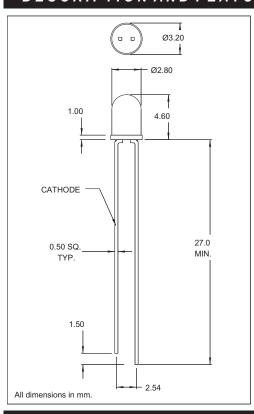
These T-1 LED lamps provide superior brightness compared to conventional LED lamps through the use of GaAIAs and improved GaP technologies. Intensities as high as 400 millicandela can be achieved with these lamps making them excellent choices for indicators in high ambient lighting conditions as well as for backlighting.
