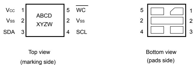
Figure 3. UFDFPN5 (DFN5) package connections
