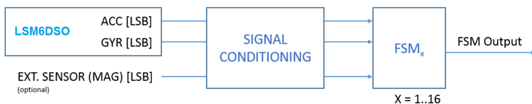
Figure 2. State machine in the LSM6DSO
