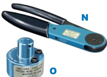
For crimping size #12 shield sleeves. These mil spec approved tools feature a ratchet mechanism to prevent damage from overcrimping. Check calibration with M22520/3 gage.
