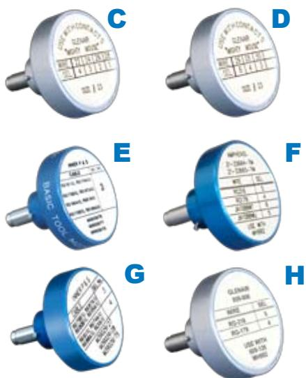
These bayonet-type positioners hold contacts at correct height for crimping with M22520/2 type miniature step adjustable tools, above. Face plate shows correct tool settings.
