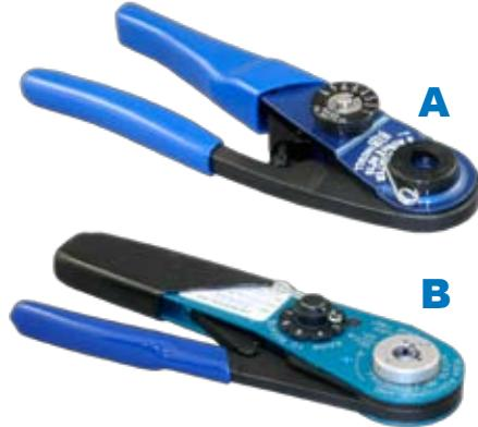
These crimp tools perform precision eight indent crimps for gas-tight wire terminations and excellent tensile strength. Adjustment wheel has 8 settings. Ratchet mechanism prevents improper crimps. Use with bayonet-type positioners. Check calibration with M22520/3 gages. Length is 6.75 inches, weight is approx. 10 oz.
