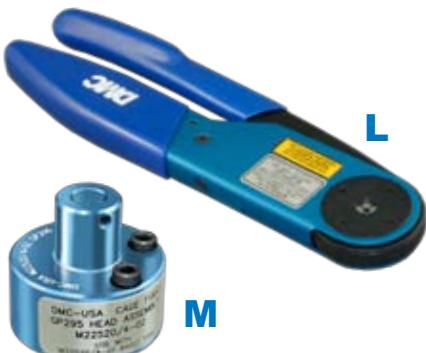
For crimping size #16 shield sleeves. These mil spec approved tools feature a ratchet mechanism to prevent damage from overcrimping. Check calibration with M22520/3 gage.
