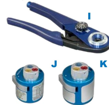
**I** Crimp tool for use with size #16 and #12 power pins. 9.75 inches OAL, 1.25 pounds. Use with M39029/57 and /58 contacts and 809-093 adapters.
