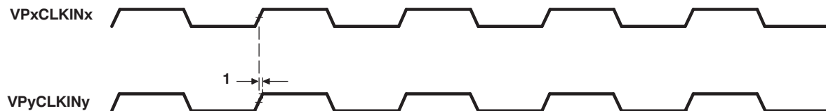
Figure 6-31. Video Port Dual-Display Sync Timing
