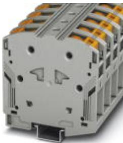
High-current terminal block, Connection method: Power-Turn connection, Cross section: 10 mm<sup>2</sup> - 70 mm<sup>2</sup>, AWG: 8 - 2/0, Width: 20 mm, Color: gray, Mounting type: NS 35/15
