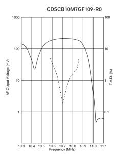
$\begin{aligned} &\text{Input} = 100 \text{dB}\mu \\ &\text{fdev.} = \pm 64 \text{kHz} \\ &\text{fmod.} = 1 \text{kHz} \\ &\text{Vcc} = 3.0 \text{V} \end{aligned}$
