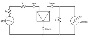
Rg+R1 =R2 : Input/Output Impedance
