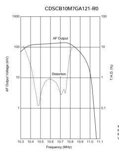
$\begin{array}{ll} \text{Input} &= 100 \text{ dB}\mu\\ \text{fdev.} &= \pm 75 \text{kHz}\\ \text{fmod.} &= 1 \text{kHz}\\ \text{Vcc} &= 3.2 \text{V} \end{array}$
