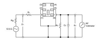
$\begin{array}{ll} Rg=50\Omega & R_1=280\Omega\pm5\% & R_2=330\Omega\pm5\% \\ C_2=10\pm2 \ pF \ (Including stray capacitance \ and Input capacitance \ of \ RF\ Volt Meter) \\ E_1: S.S.G. \ Output \ Voltage \end{array}$
