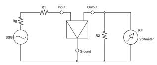
Rg+R1 =R2 : Input/Output Impedance
