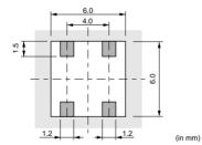
The material of P.C.B. is the epoxy resin of glass fabric base (t=0.8mm)
