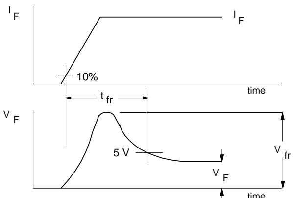
Fig. 3. Definition of anti-parallel diode  $V_{fr}$  and  $t_{fr}$ .
