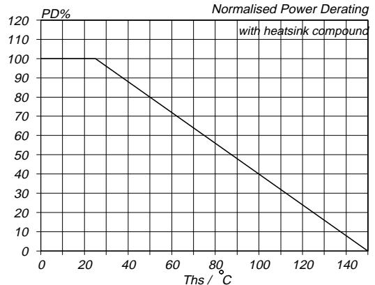
Fig.10. Normalised power dissipation.
