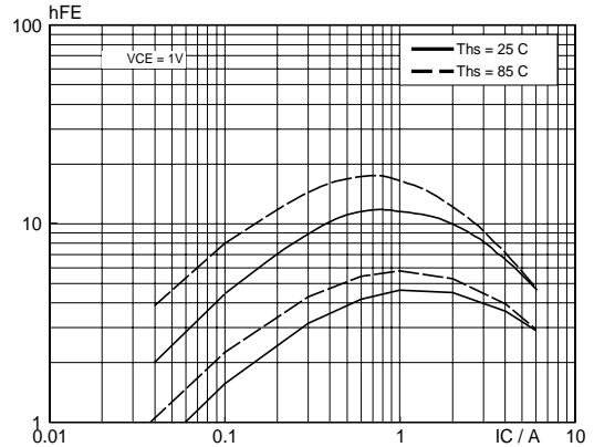
Fig. 5. High and low DC current gain.
