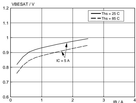
Fig.8. Typical base-emitter saturation voltage.
