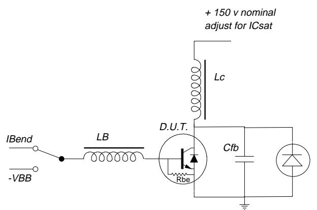
Fig. 4. Switching times test circuit.
