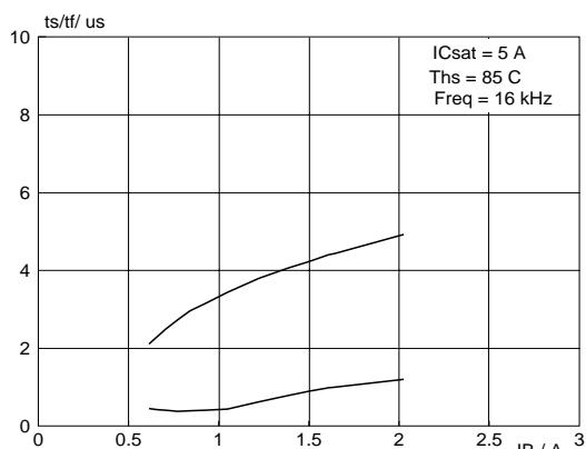
Fig.9. Typical collector storage and fall time.
