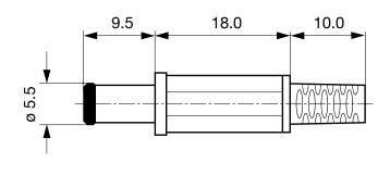
Cable diameter max. 4.0 mm
