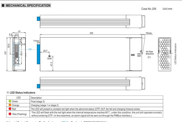
※ Input / Output Connector Pin No. Assignment(CN1): Positronic PCIM34W13M400A1
