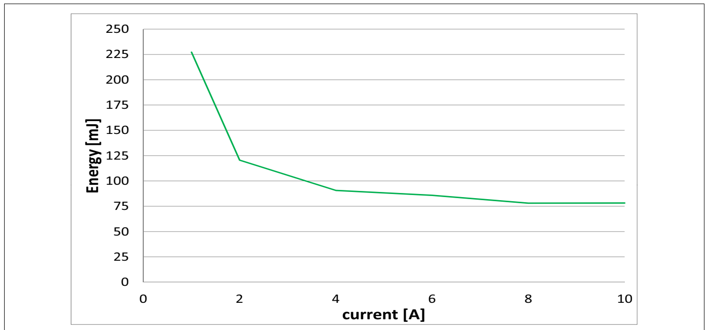
Figure 12 Maximum Energy Dissipation Single Pulse, T_{J(0)} = 150 \text{ }^\circ\text{C} ; V_S = 28 \text{ V}
