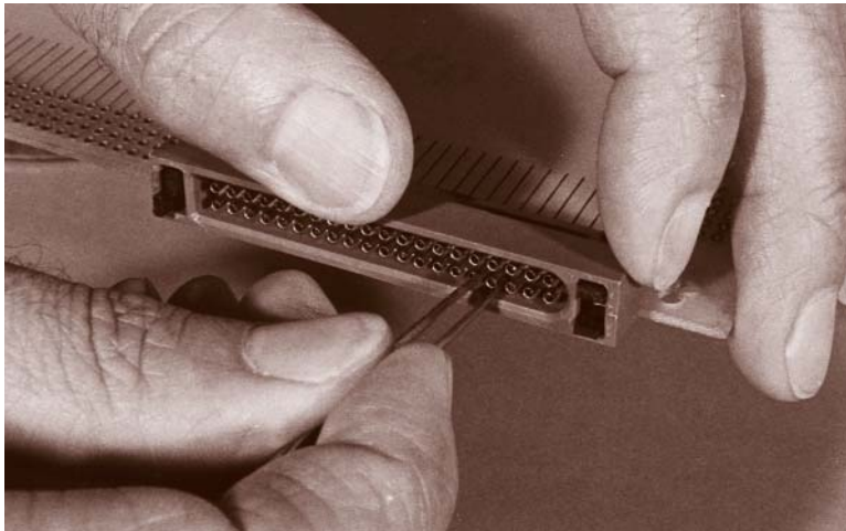
REMOVE DAMAGED CONTACT
