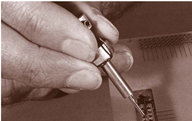
INSERT EXTRACTION TOOL WITH PLUNGER RETRACTED
