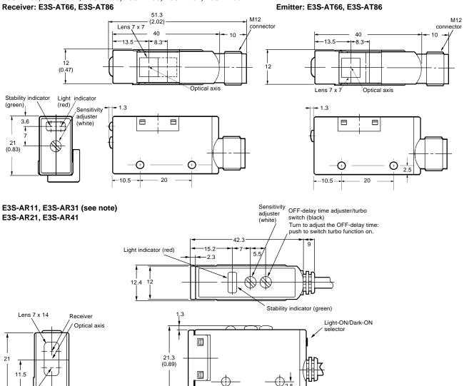
NOTE: No time adjuster/turbo included on models E3S-AR11 and E3S-AR31.
