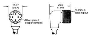
2 m (6.56 ft) length for Y96E-43RD2 5 m (16.40 ft) length for Y96E-43RD5 10 m (32.81 ft) length for Y96E-43RD10
