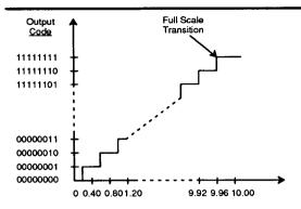
Input Voltage, Volts (Referred To Analog Ground)
