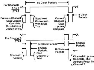
Figure 3. STAT Output for Channel Identification
