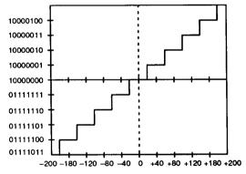
Input Voltage, Millivolts (Referred to Analog Ground)
