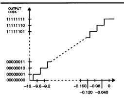
Input Voltage, Volts (Referred to Analog Ground Note: Approximate Bit Weights are Shown for Illustration. Bit Weight for a -10 V Reference is ~ 39.1mv.
