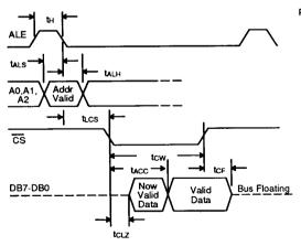
Figure 2. Timing Diagram for the MP7581
