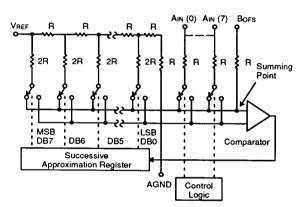
Figure 1. D/A Converter as used in the MP7581
