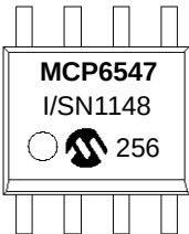
8-Lead SOIC (150 mil) (MCP6546, MCP6547, MCP6548, MCP6549)
