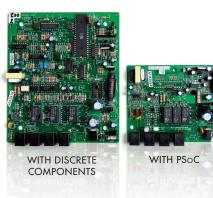
INTEGRATION: In this communications product, PSoC technology reduced the BOM from 12 ICs to 3 by integrating FSK detection, voltage monitoring, DTMF, and ringtone generation.
