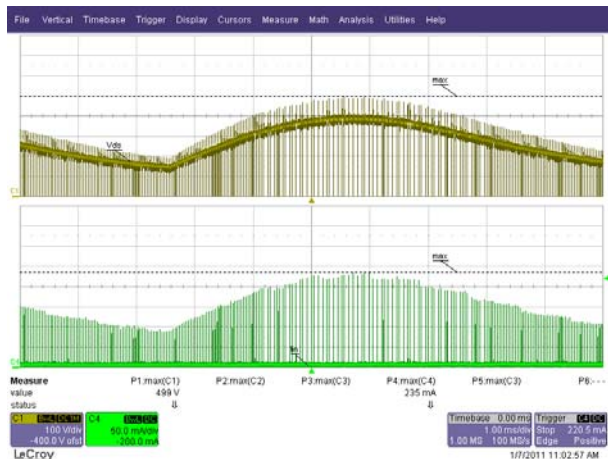
Figure 35 – 265 VAC. Load Shorted. Upper: V_{DRAIN} , 100 V / div. Lower: I_{DRAIN} , 50 mA / div., 1 ms / div.
