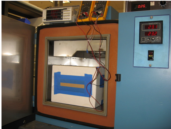
Figure 19 – Thermal Chamber Set-up Showing Box Used to Prevent Airflow Over UUT.
