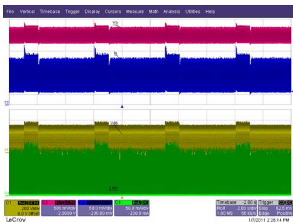
Figure 61 – 230-265-230 VAC / 50 Hz. LED = 3 V / 366 mA. Ch1(Yellow): V_{DS} , 200 V / div. Ch2(Red): V_{IN} , 0.5 V / div. Ch3(Blue): I_O , 100 mA / div. Ch4(Green): I_{DS} , 50 mA / div., 2 s / div.
