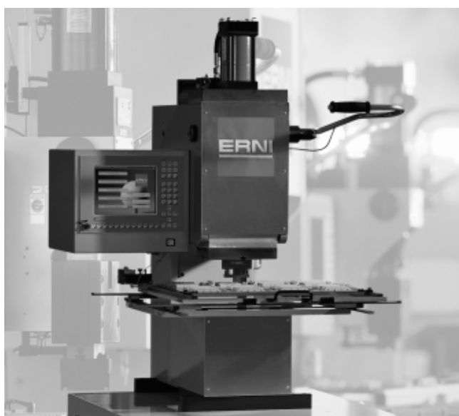
EPC 24 ERNIPRESS CENTER Hydro Pneumatic Press With Industrial PC For Network Integration
