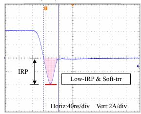
Conditions: FCC 160kHz Load 5A (DC12V)
