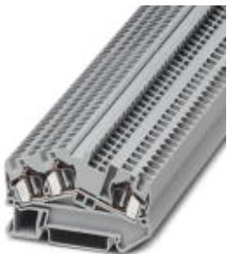
Feed-through terminal block, Connection method: Spring-cage connection, Cross section: 0.08 mm<sup>2</sup> - 6 mm<sup>2</sup>, AWG: 28 - 10, Width: 6.2 mm, Color: orange, Mounting type: NS 35/7,5, NS 35/15
