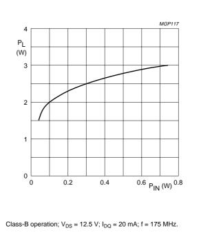
Fig.9 Load power as a function of input power; typical values.
