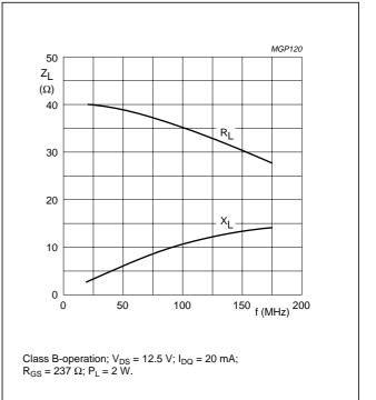
Fig.12 Load impedance as a function of frequency (series components); typical values.
