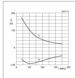
Class B-operation; V<sub>DS</sub> = 12.5 V; I<sub>DQ</sub> = 20 mA; R<sub>GS</sub> = 237  $\Omega$ ; P<sub>L</sub> = 2 W.
