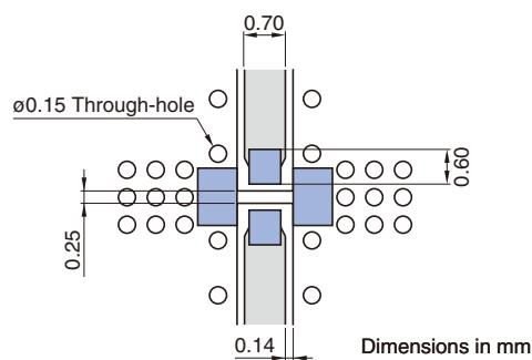
Line width be designed to match 50Ω characteristic impedance depending on PCB material and thickness.
