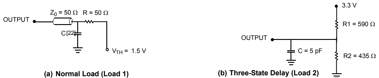
Figure 3. AC Test Loads and Waveforms
