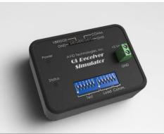
The Qi FOD Receiver is a power receiver that can be placed on Qi wireless transmitters and used to test the operation and FOD performance. DIP switches on top of the FOD Receiver are used to program received power offsets and to change internal loads.
