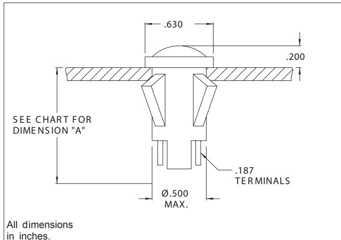
Mounting: Will snap-fit into Ø.500/.505 hole in panels .020/.100 thick. Push-on speednut SN0461 also available. Mounting hole pattern on page SP2.
