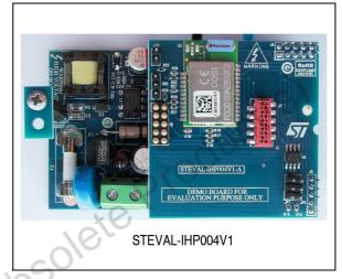
The current, power, energy and other info related to the electrical load connected to the smartplug board are sent to an IEEE-802.15.4 data concentrator through the home/building RF network.
