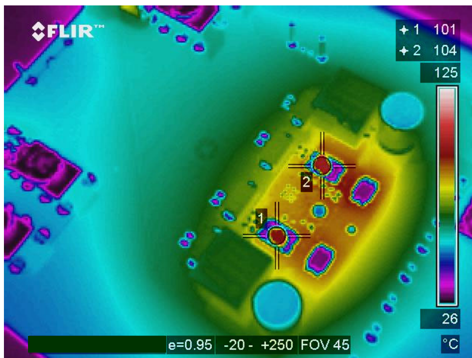
Fig. 40: Thermal Image at 60 A load, without heatsink, and with no air flow, Test Points are Synchronous Rectifier DirectFETs.
