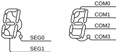
Figure 15-6 Example of COM, SEG Pin Connection (1/4 Duty)
