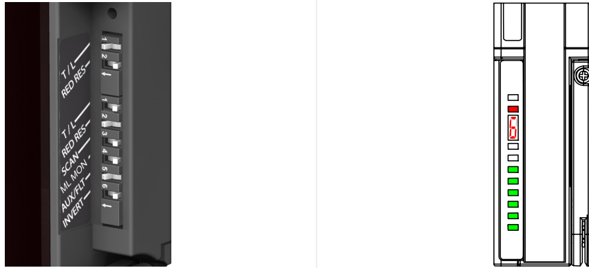
Figure 23. DIP switch settings to program mute configuration options
