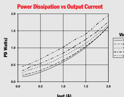
**Note 1:** All data listed in the above graphs, except for derating data, has been developed from actual products tested at 25°C. This data is considered typical data for the ISR.
