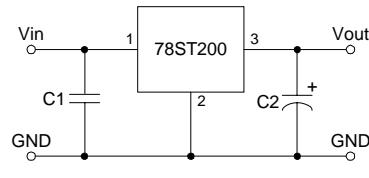
C1 = Optional 1 $\mu$ F ceramicC2 = Required 100 $\mu$ F electrolytic
