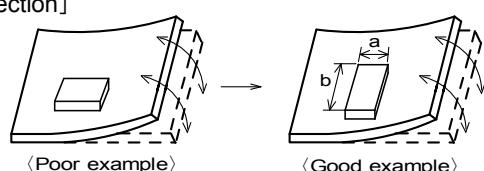
Products shall be located sideways direction (Length:a<b) to the mechanical stress.
