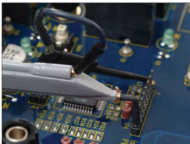
Use the Right-angle Connector and the Sprung Hook to probe square pins spaced far apart from each other.
