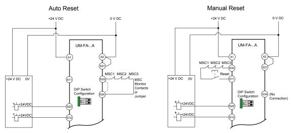
Single-Channel Wiring Configuration for Devices with Hard Contacts
