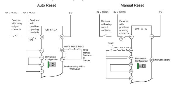
Single-Channel Wiring Configuration for Solid State Devices
