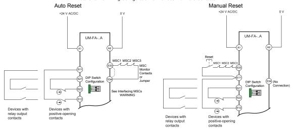
Dual-Channel Wiring Configuration for Solid State Devices (+24 V DC Supply Only)
