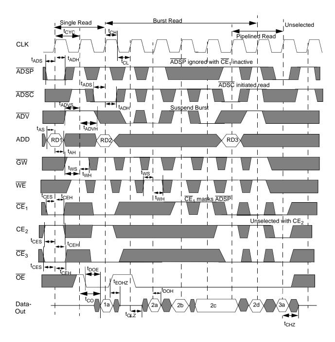
$\overline{\text{WE}}$  is the combination of  $\overline{\text{BWE}}$  &  $\overline{\text{BW}}_{\text{X}}$  to define a write cycle (see Write Cycle Descriptions table).
