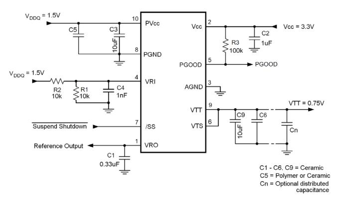
Figure 1. Standard Application Schematic for NCP51510
