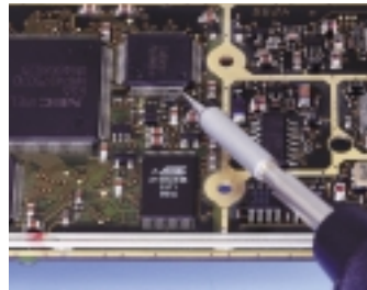
SMD-soldering with the Micro tool
