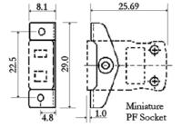
Recommended aperture size and hole pitch for panel mounting
