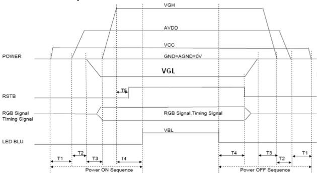
Note: T1≥20ms, T2≥20ms, T3≥5ms, T4≥100ms, T5≥5ms.
