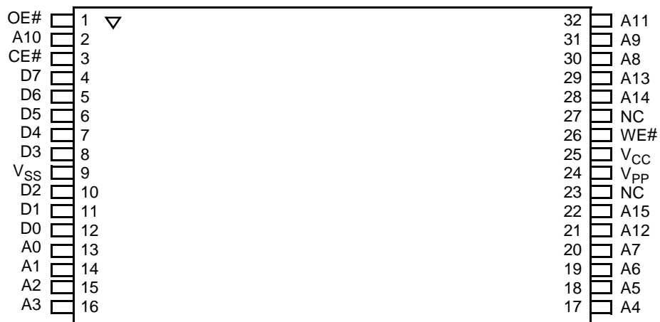
32-Pin TSOP—Reverse Pinout
